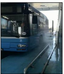
**PURPOSE:** high pressure skirt wash will spray 150 bars high pressure water on the skirt sides to remove dirt over the wheel and skirts
