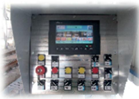
Showing Failures and remedies, showing washing numbers, make adjustments for brush pressure control.
