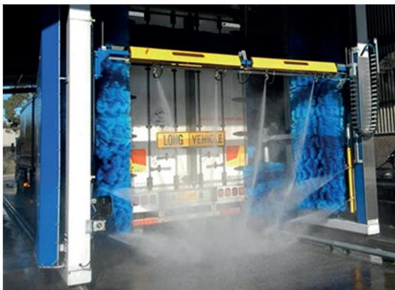
The high pressure washing system consists of one chemical dosage and spray group, Side high pressure up and down oscillating impact nozzle spray group and one top high pressure automatic profile following nozzles group with possibility of tilting to the vehicle face during washing.
