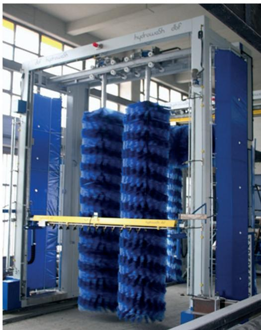
As the side brushes approach to the vehicle, in the first sensing of the brush pressure, the gantry retracts to allow the soft side movement of the side brushes and then approach again.
